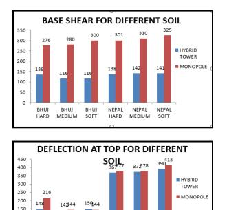
HARD Fig. 4. Comparison of base shear and displacement for monopole and hybrid tower in different soil conditions
